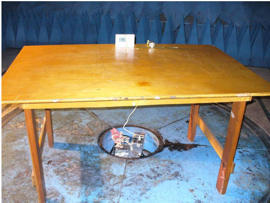
Photographs 3 & 4: Radiated Emission Setup
