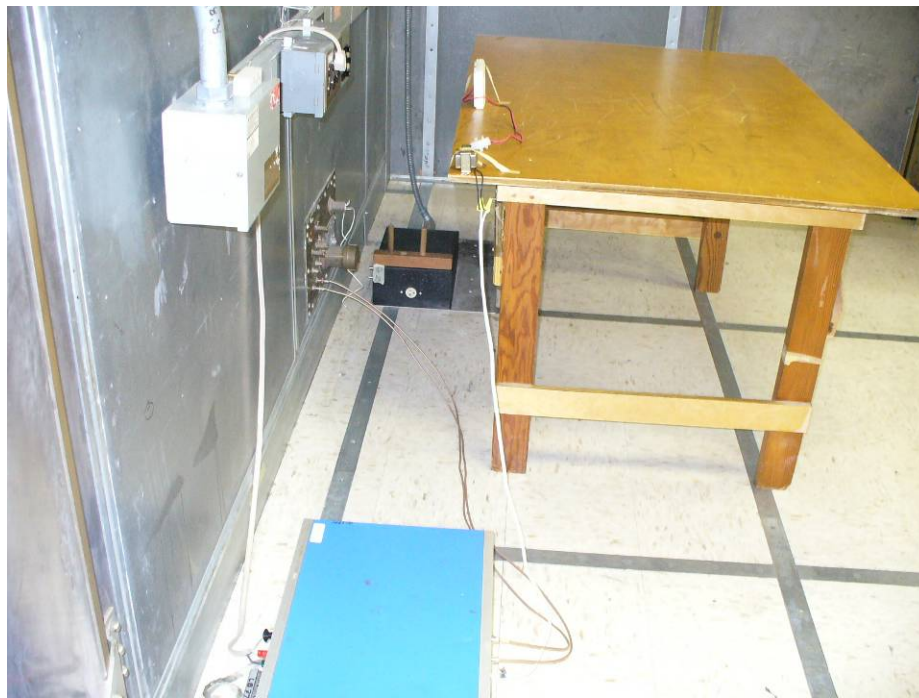
Photographs 1 & 2: Conducted Emission Setup
