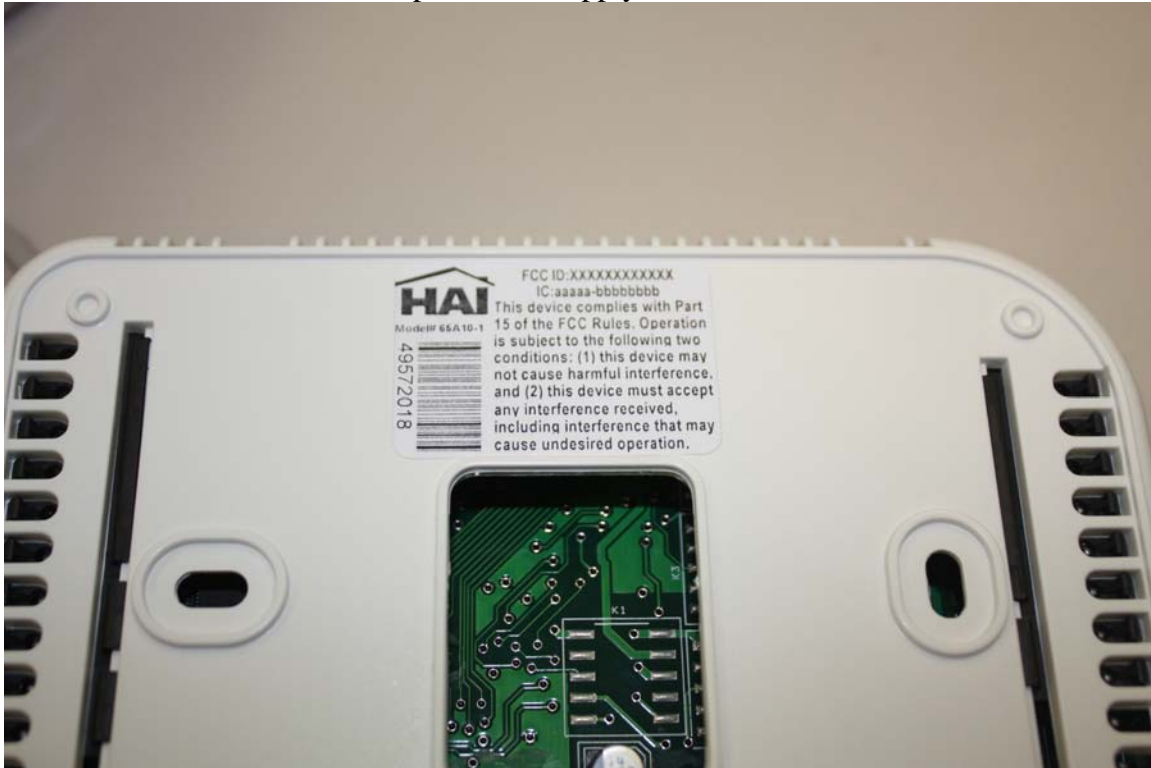
Example of label attached to an HAI 65A01-1 Omnistat2 (Thermostat)
