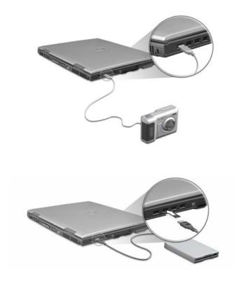
USB is plug and play, which means that you can connect and start using a USB device without having to restart your computer. You can also disconnect the device at any time.
