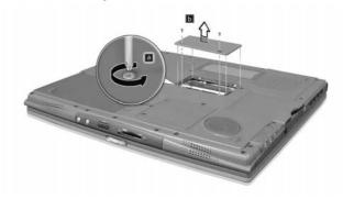
3 Insert the memory module diagonally into the slot (a), then gently press it down (b) until it clicks into place.
