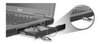
When the power is off, you can eject the drive tray using the emergency eject hole. See page 58.
