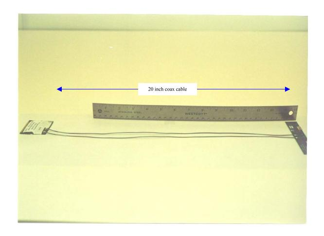
Cable Length Between Antenna and Device "Ethertronics Antennas"
