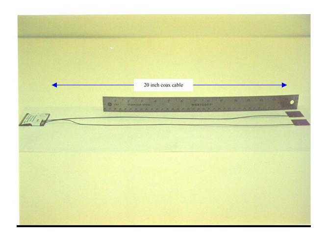
Cable Length Between Antenna and Device "Hitachi Antennas"
