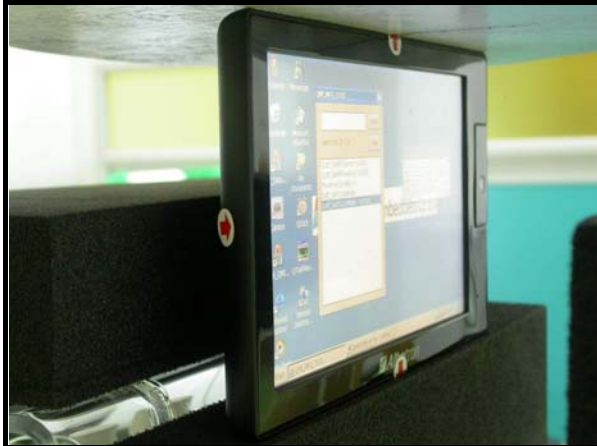
A. The edge of the EUT face to the phantom with 0mm-separation distance.
