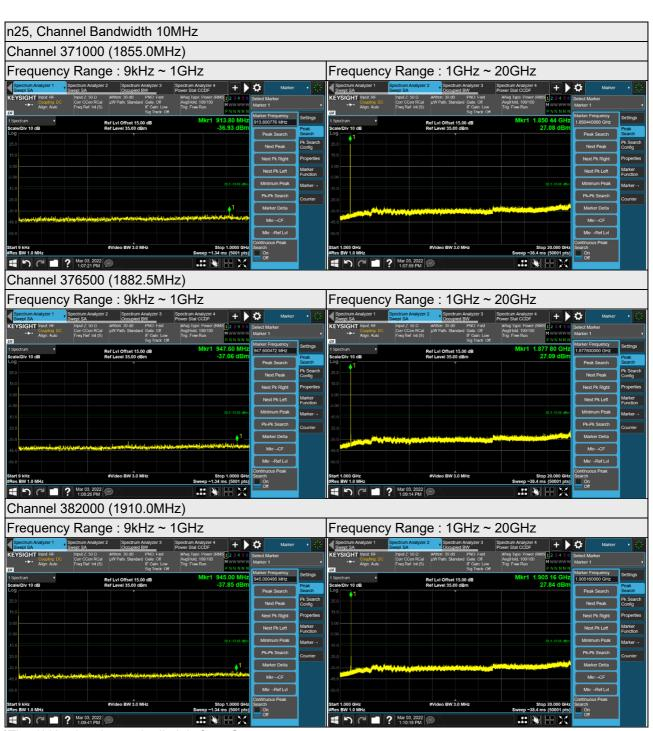
\*The 9kHz signal over the limit is from Spectrum.
