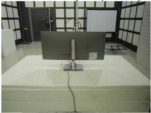
Radiated Emission Set up Photos (Below 1GHz)
