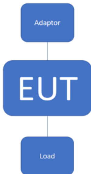
Fig. 2-1 Conduction & Radiated Emission test set up configuration
