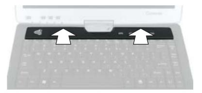
**6** Press down on the bezel in several places to make sure it is correctly mounted. The bezel is correctly mounted when you can run you finger along the bezel and find no loose spots. The bezel should be flat all the way across.
