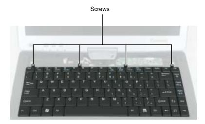
**11** Lift the back edge of the keyboard, then slowly rotate it toward you so it lies **keys-down** on top of your convertible tablet PC. Be careful not to damage the LCD panel.
