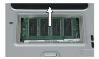
**9** Hold the new or replacement module at a 30-degree angle and press it into the empty memory slot. This module is keyed so it can only be inserted in one direction. If the module does not fit, make sure that the notch in the module lines up with the tab in the memory bay.
