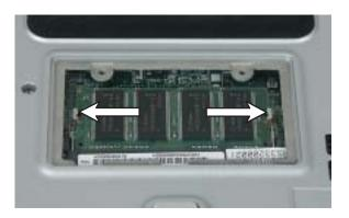
**8** Pull the memory module out of the slot.
