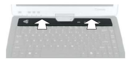
**6** Press down on the bezel in several places to make sure it is correctly mounted. The bezel is correctly mounted when you can run you finger along the bezel and find no loose spots. The bezel should be flat all the way across.
