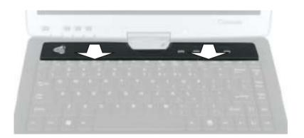
**10** With a small Phillips screwdriver, remove the four keyboard screws and put them in a safe place.
