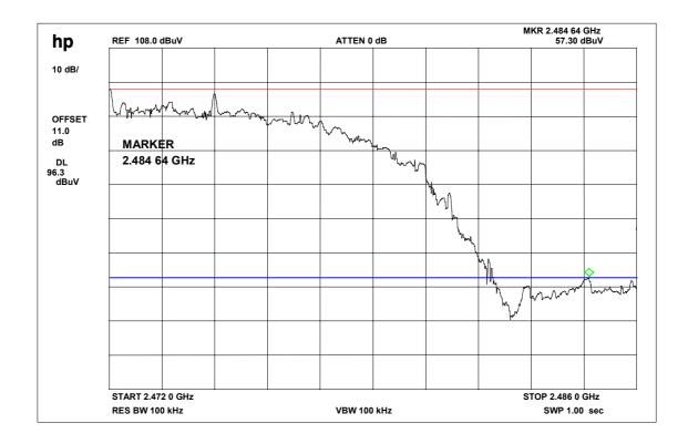
The range is from middle carrier highest frequency up to 2Mhz into restricted band. Span is 14 MHz, so we choose a RBW of 1% span, here 100 kHz.
