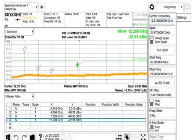
Spurious Emission_BLE 1M_MidCH20-2442MHz
