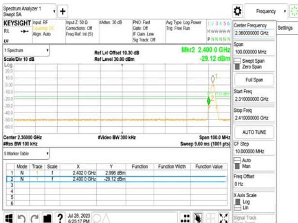
Band Edge_BLE 2M_LowCH00-2402MHz
