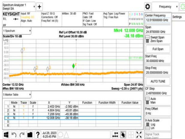
Spurious Emission_BLE 2M_MidCH20-2442MHz
