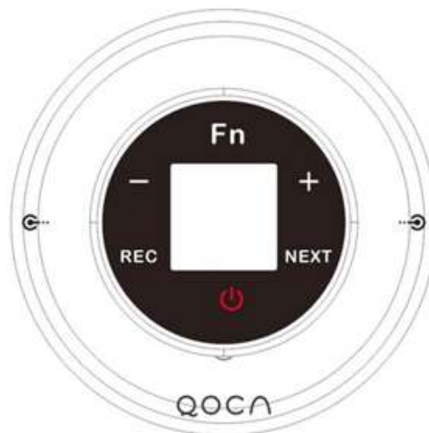
Figure 2. The top view of QOCA digital stethoscope showing the location of six touch keys
