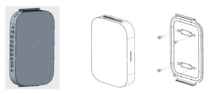
Find the 'Pill Shape' marking to orientate the box so that the exhaust/fan faces upwards
