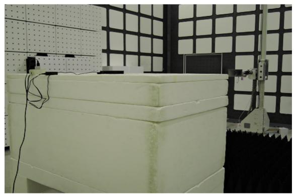
Radiated Emission Set up Photos (Front View)
