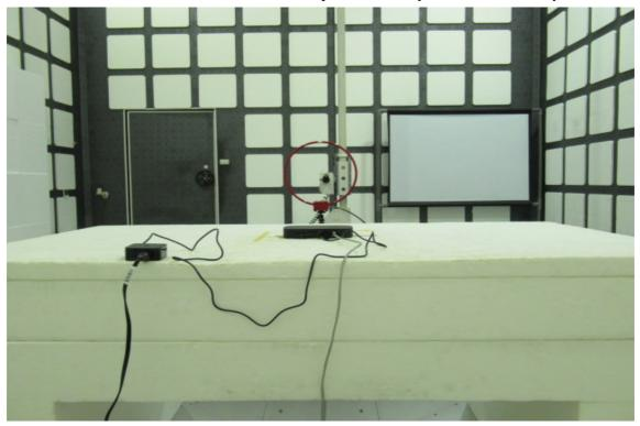
Radiated Emission Set up Photos (Below 1GHz)
