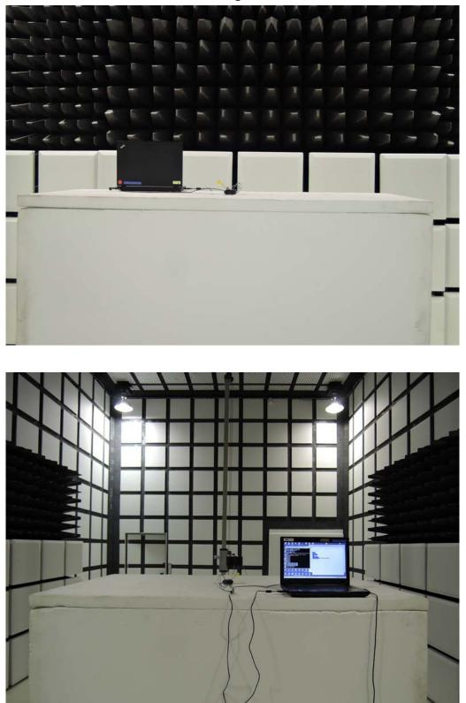
**Radiated Emission Set up Photos (Above 1GHz)**
