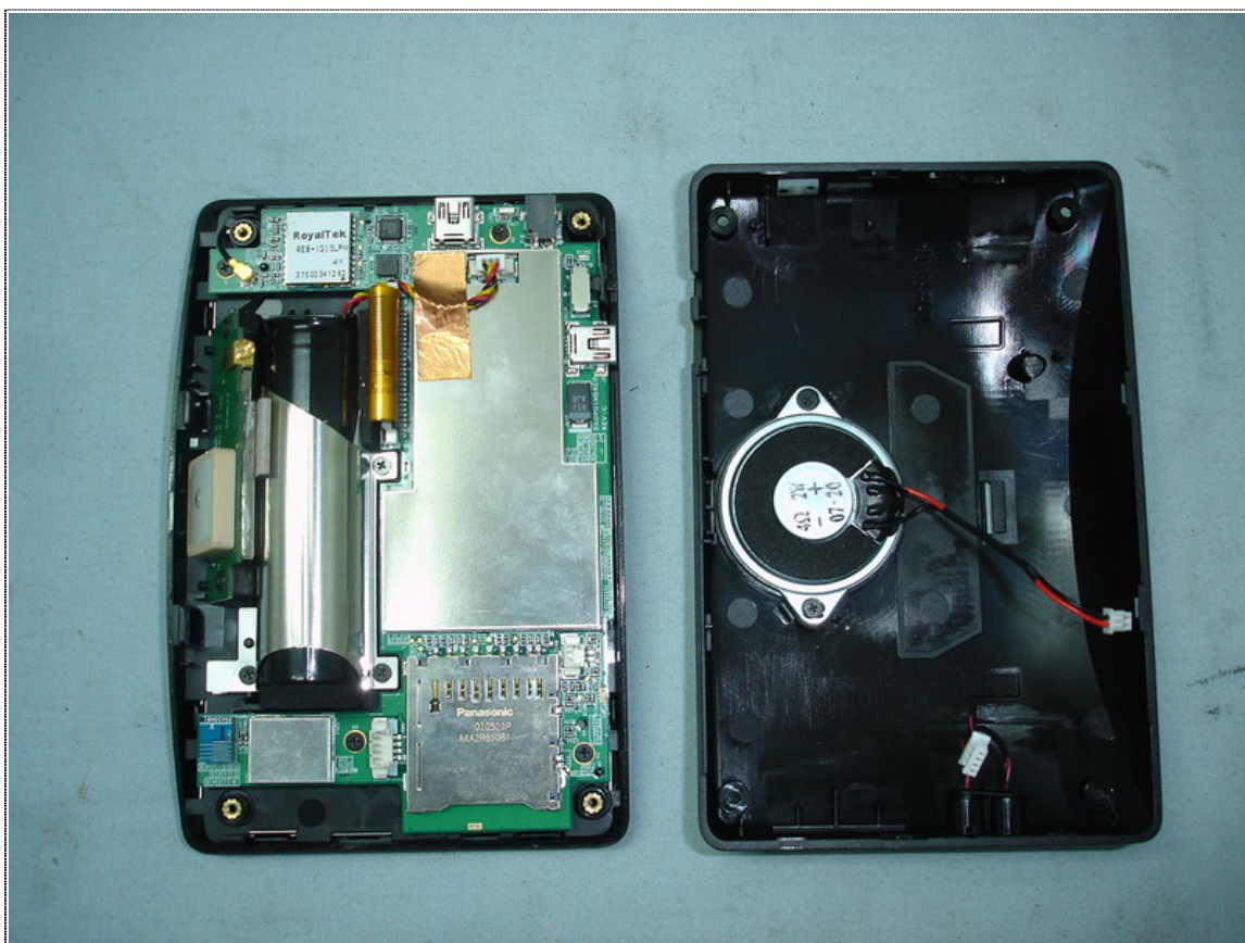
Inner View of EUT-1
