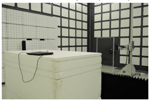
Radiated Emission Set up Photos (Front View)
