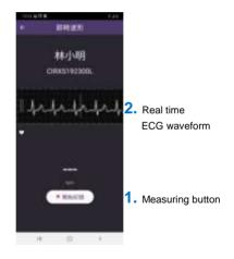
Once you tap the measuring button, it will start taking ECG measurement for 2 minutes. And you could see the countdown time bar is counting.
