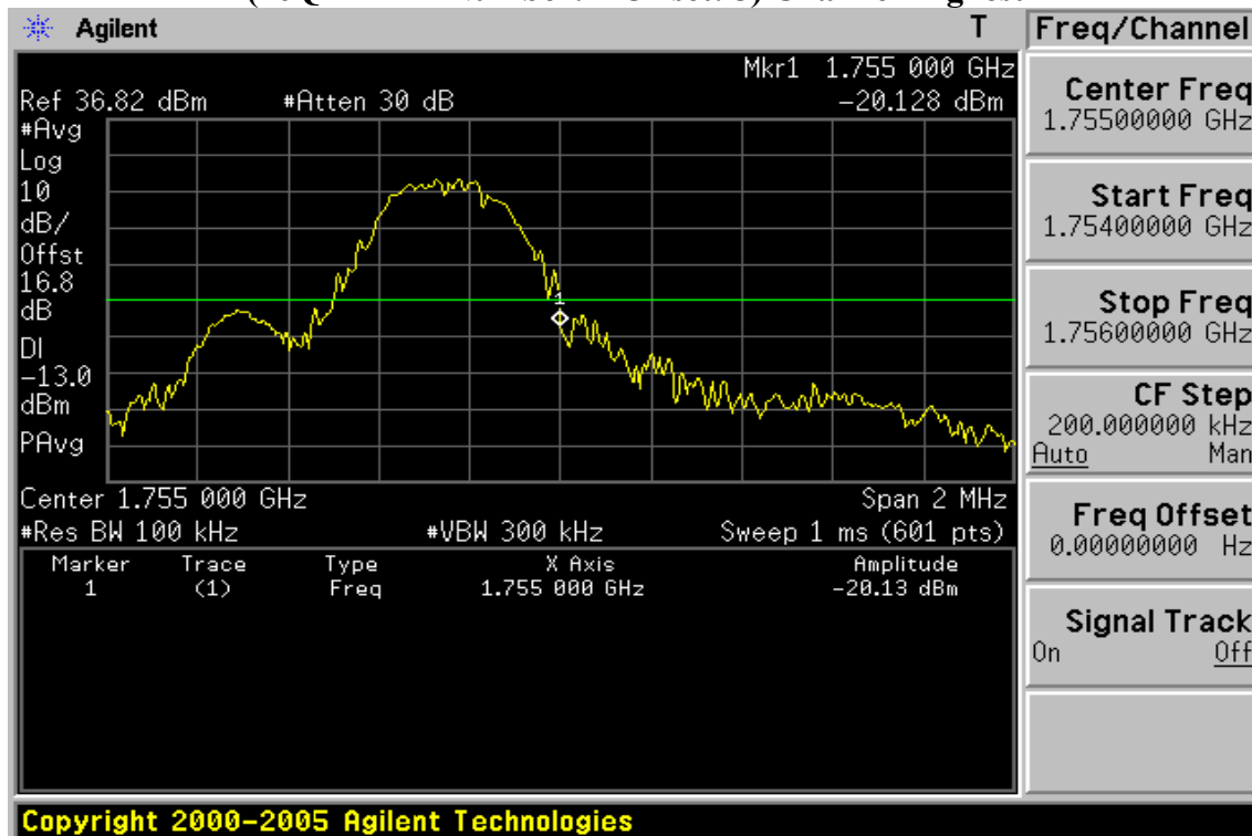
Figure 10-55: Band edge emission at antenna terminals –1.4MHz BW LTE-Band 4 (16QAM RB Number: 1 Offset: 5) Channel Highest
