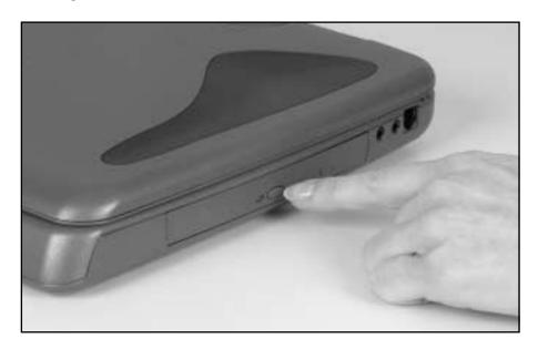
**2** Place the CD in the tray with the label up, then press down carefully on the disc until it snaps into place.
