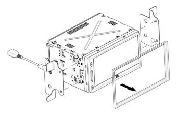
Brackets and faceplate are vehicle specific and are customer provided
