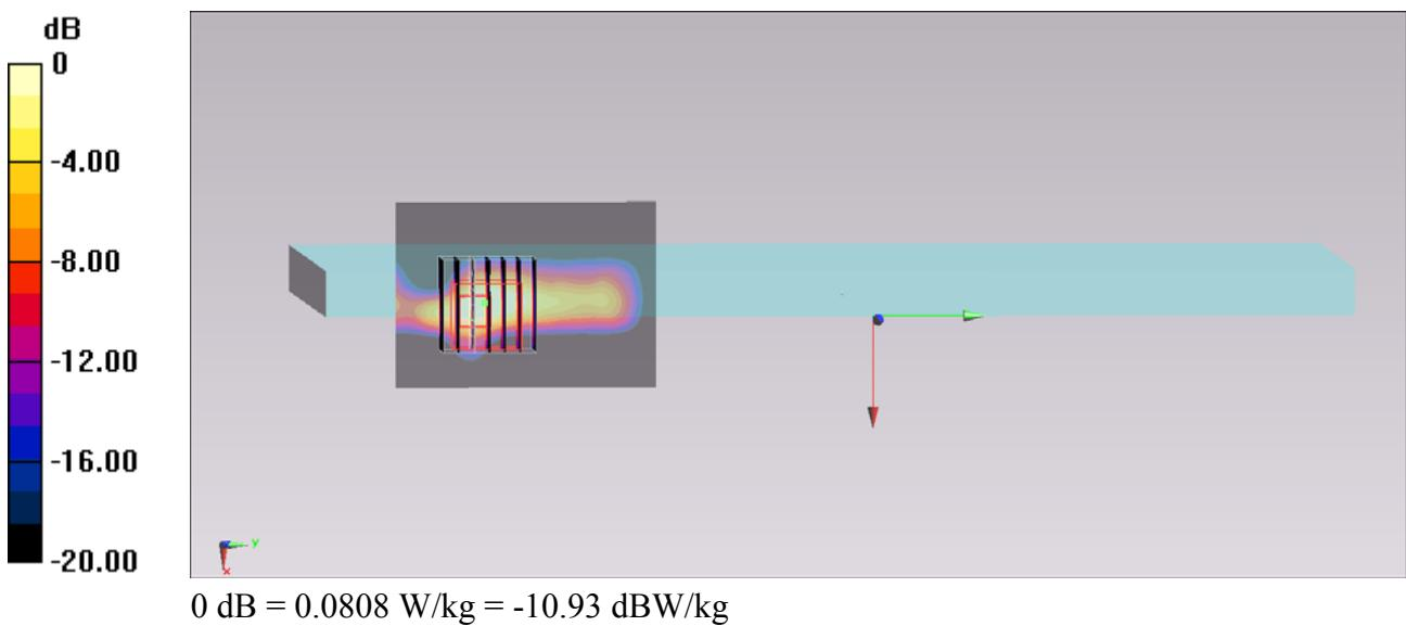
**#152\_WLAN2.4GHz\_802.11b 1Mbps\_Curved surface of Edge1\_0cm\_Ch6;Ant 2**
