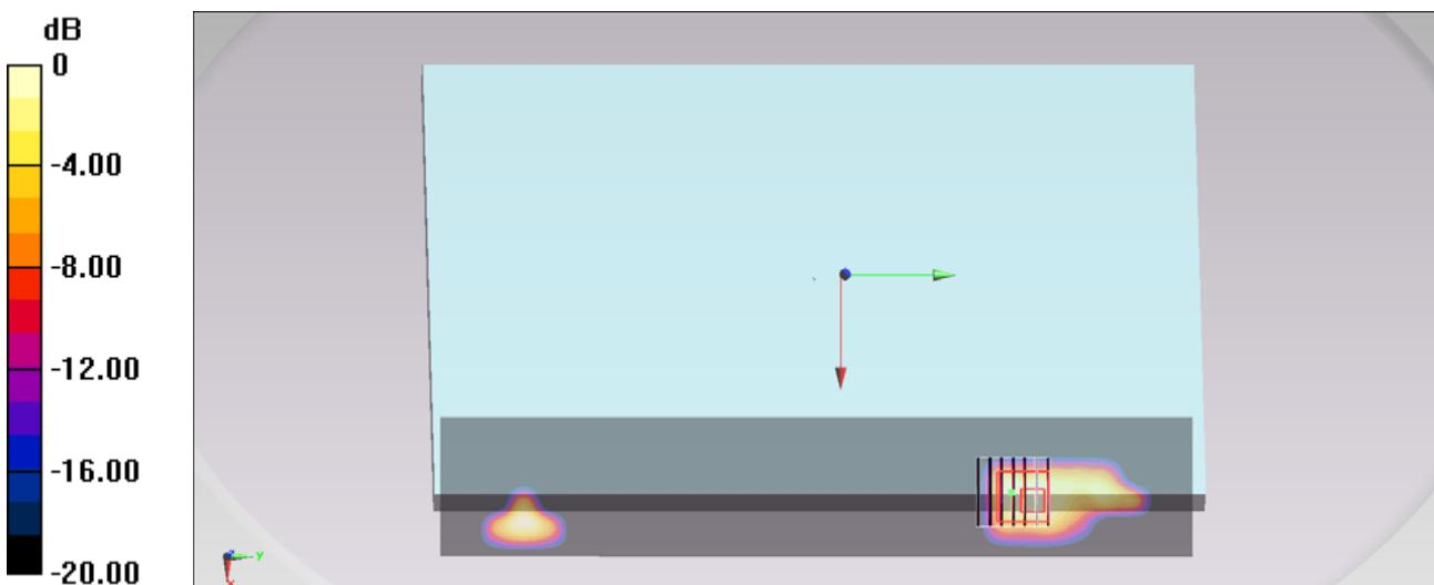
**#166\_WLAN5GHz\_802.11a 6Mbps\_Bottom Face\_0cm\_Ch40;Ant 1**
