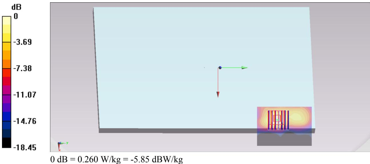
**#147\_WLAN2.4GHz\_802.11g 6Mbps\_Curved surface of Edge1\_0cm\_Ch6;Ant 1**
