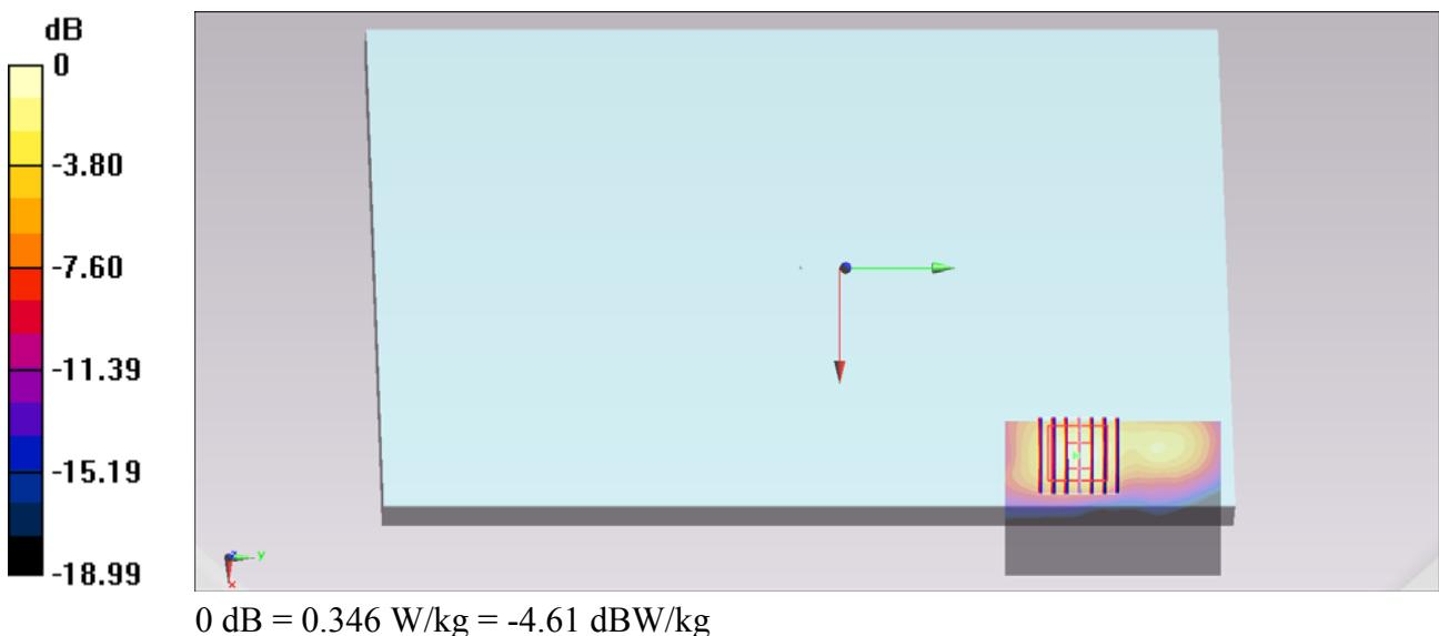
**#148\_WLAN2.4GHz\_802.11n-HT20\_Curved surface of Edge1\_0cm\_Ch6;Ant 1**
