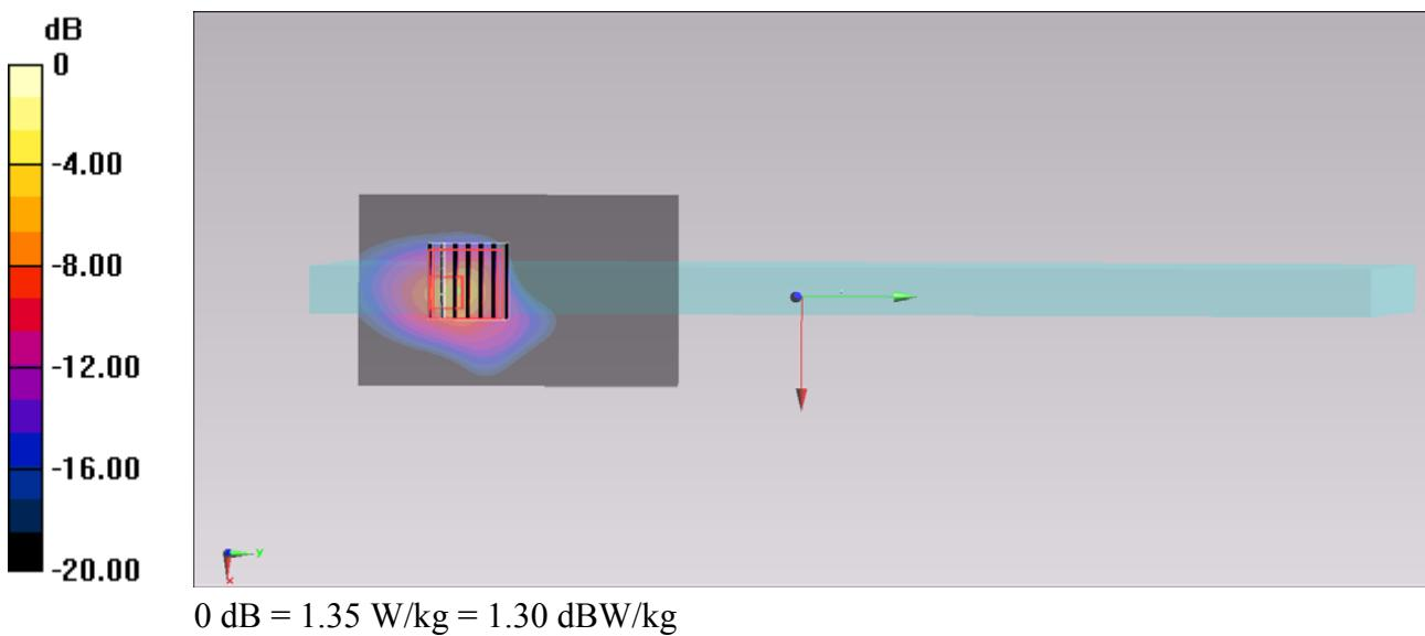
**#175\_WLAN5GHz\_802.11a 6Mbps\_Bottom Face\_0cm\_Ch56;Ant 2**
