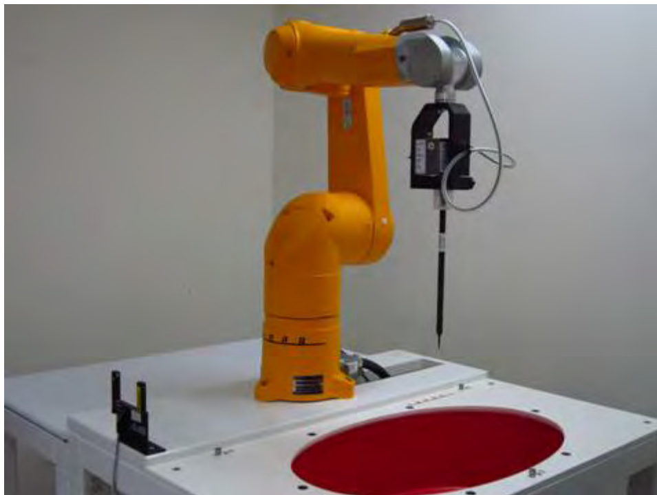
Fig.1 Photograph of the SAR measurement system
