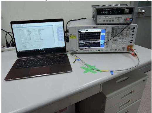
**Conducted Setup Photo (Measurement at Antenna Port)**
