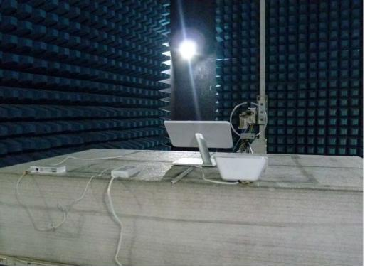
Radiated Emission Setup Photos (30MHz~1GHz)
