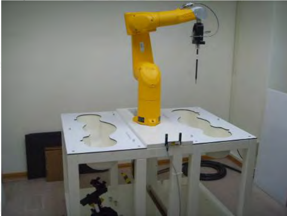
Fig.1 Photograph of the SAR measurement System
