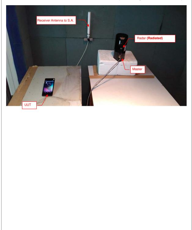
Set UUT as Client without radar detection mode (Radar injected into Master)
