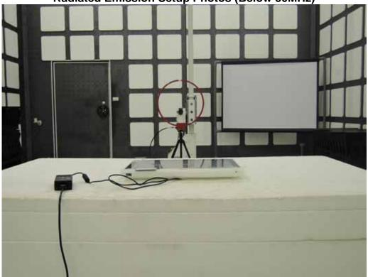
Radiated Emission Setup Photos (Below 1GHz)
