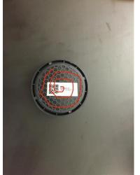
• Put high viscosity (HV) adhesive around the outside of the ring. Put the ring down around the sensor and stand on it
