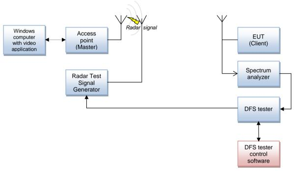
Figure: 1 Test setup DFS test for slave devices
