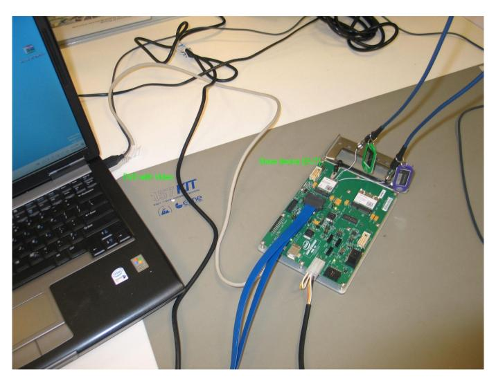
EUT setup with laptop and DVD with Video. The video is displayed via the RF connection to the Access Point on a second laptop
