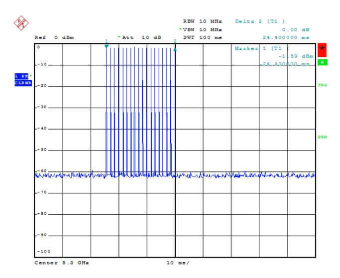
Figure: 2 Radar burst
