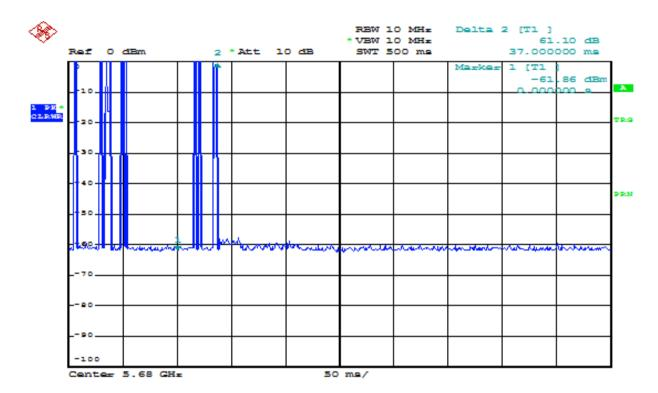
Channel Closing Time - Radio channel 5680 MHz (Marker 1 represents end of the radar pulse)
