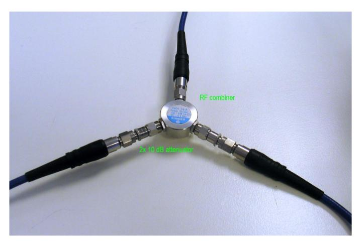
Combiner and 2x 10 dB attenuator to combine the two antenna ports of the EUT. The output of the combiner is connected to the spectrum analyzer. The If output of the spectrum analyzer is connected to the DFS testtool.
