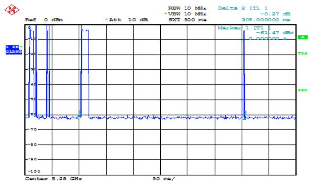
Channel move time (Marker 1 represents end of the radar pulse)
