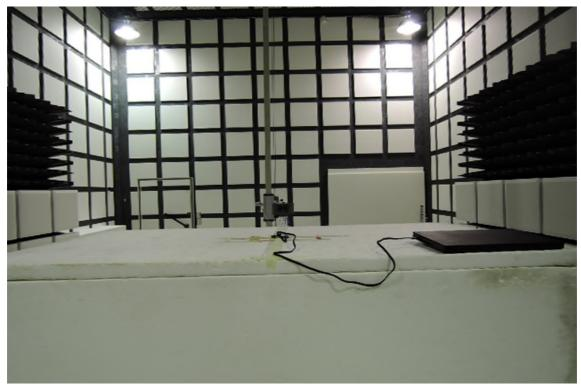
Radiated Emission Set up Photos (Front View)
