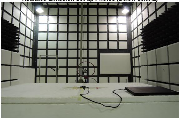
Radiated Emission Set up Photos (Below 1GHz)
