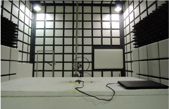
Radiated Emission Set up Photos (Below 1GHz)
