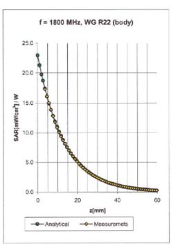
Body 900 MHz  $\epsilon_r = 55.0 \pm 5\%$  $\sigma$  = 1.05 ± 5% mho/m Valid for f=800-1000 MHz with Body Tissue Simulating Liquid according to OET 65 Suppl. C  $6.5 \pm 9.5\% (k=2)$ ConvF X Boundary effect: ConvF Y  $6.5 \pm 9.5\% (k=2)$ 0.31 Alpha ConvF Z 6.5 ± 9.5% (k=2) 2.92 Depth 1800 MHz  $\varepsilon_r$  = 53.3 ± 5%  $\sigma$  = 1.52 ± 5% mho/m Body
