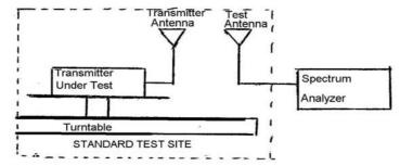
b) Raise and lower the test antenna from 1m to 4m and rotate turntable from 0° to 360°. Record the highest received signal showed in spectrum analyzer as Rt . Calculate electric field strength in receive antenna as Et.
