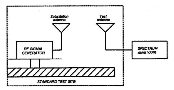
Name of Test: Field Strength of Spurious Radiation (Cont.)
