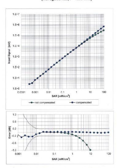
Dynamic Range f(SAR<sub>head</sub>) (Waveguide R22, f = 1800 MHz)
