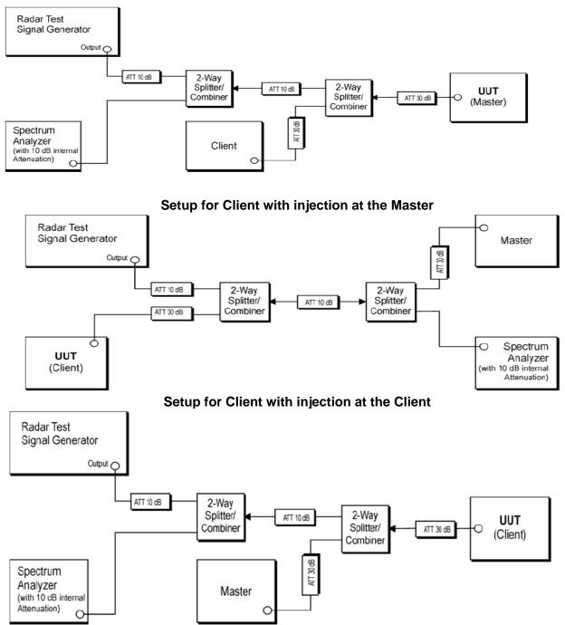
Setup for Master with injection at the Master
