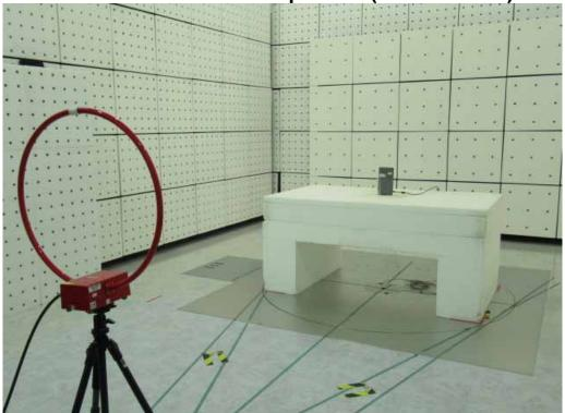
Radiated Emission Set up Photo (Below 1GHz)
