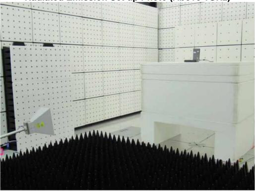
Radiated Emission Set up Photo (Front View)
