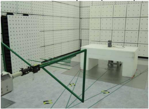
Radiated Emission Set up Photos (Above 1GHz)
