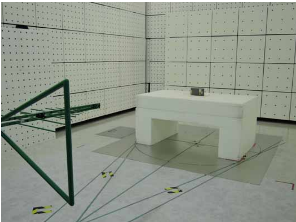
Radiated Emission Setup Photos (30MHz~1GHz)
