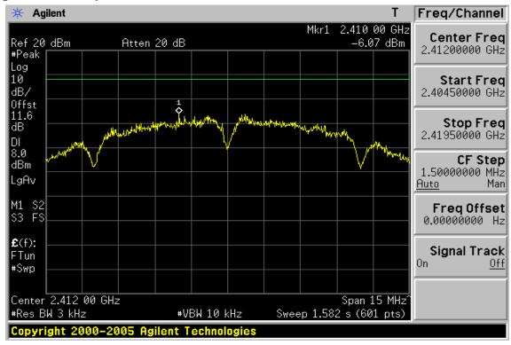
**Power Spectral Density Test Plot (CH-Mid)**
