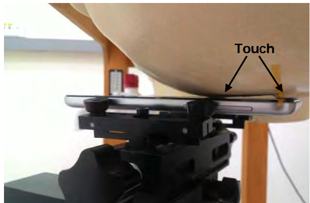
Fig.5 Left Head Section / Cheek-Touch Position
