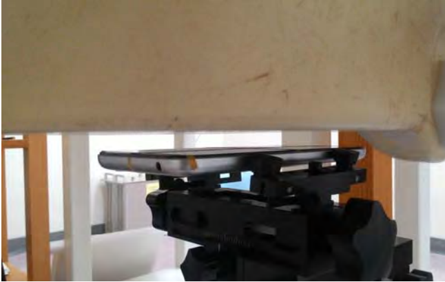
Fig.8 EUT front side to flat phantom
