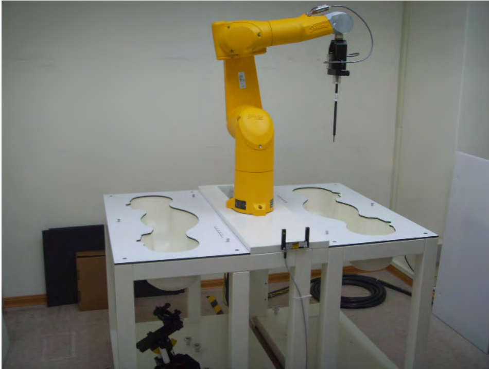
Fig.1 Photograph of the SAR measurement system
