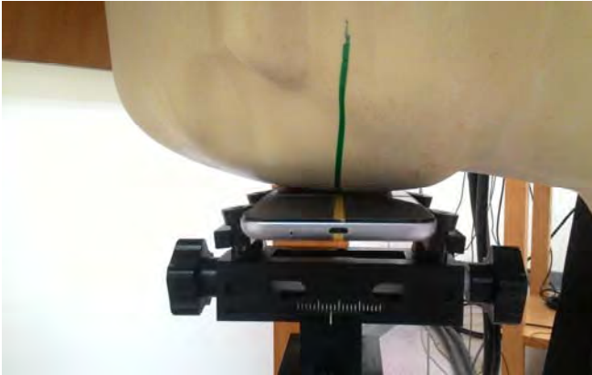
Fig.3 Right Head Section / Cheek-Touch Position
