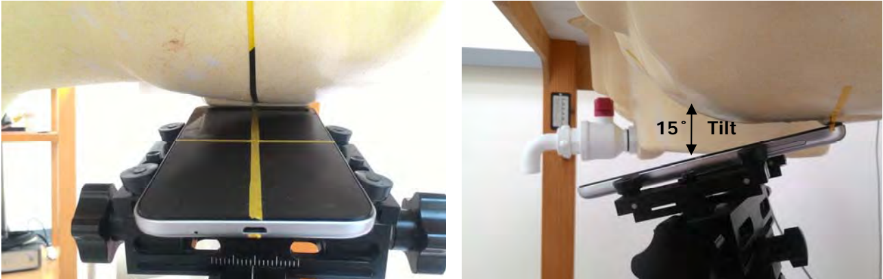
Fig.6 Left Head Section / Ear-Tilt Position(15°)
