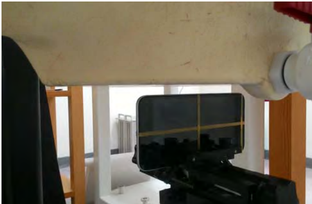
Fig.13 EUT left to flat phantom
