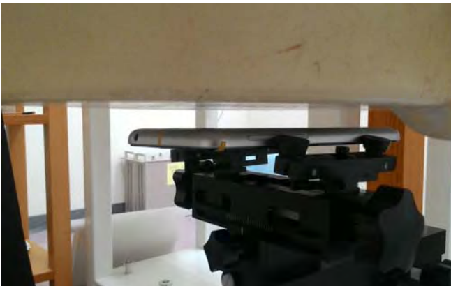
Fig.9 EUT back side to flat phantom
