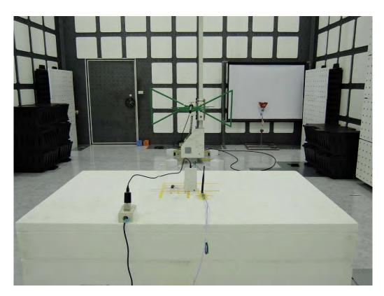
Radiated Emission Set up Photos E1 plan (Below 1GHz)
