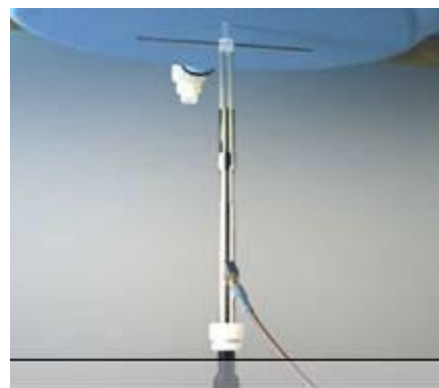
Photograph of the Dipole Antenna
