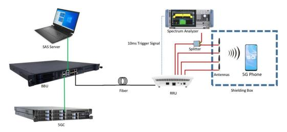
E2E test signal config: power setting 18dBm/port, 24dBm/4 ports
