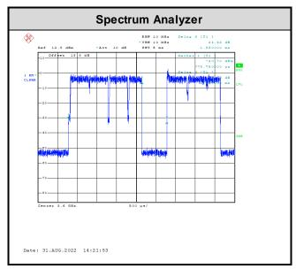
Note: The duty cycle value is 74.4%, add 10log(1/duty cycle) to the measured power level to compute the average power during continuous transmission.
