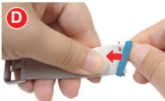
5. Insert the pin (the opposite side of the release knob) into the pin hole on your GizmoWatch (E).
