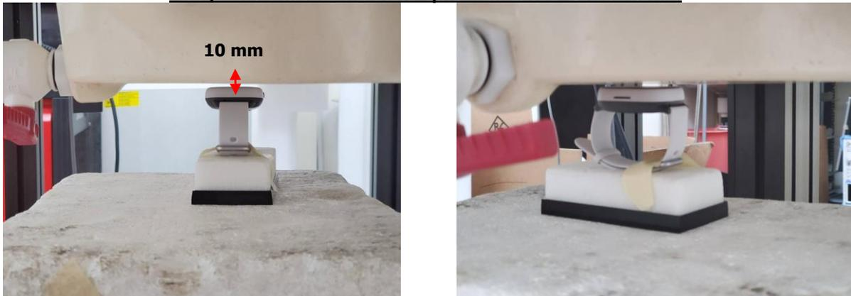
**Fig.4 Front side of EUT to flat phantom**
